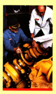
QUALITY CONTROL: Ongoing quality assurance/control is essential to maintain product reliability. Here, a Quality Control inspector measures a critical point of the pump volute. Hydrostatic tests are performed in accordance with Hydraulic Institute Standards.
